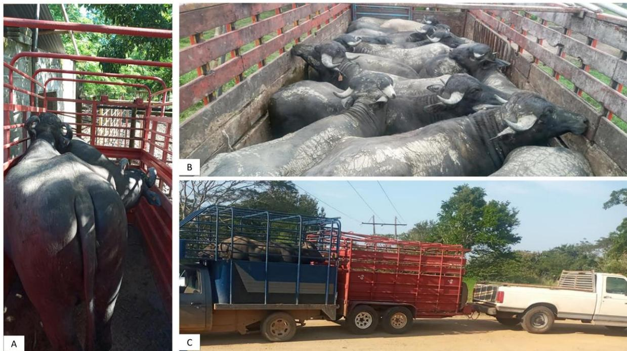
**Figure 4** (A) and (B) load density and type of vehicle used to transport water buffaloes with upper tubular structures at least 30 cm above the height of the animals (dimensions recommended by the FAWC, 2019). (C) comparison of vehicles used for transport. Regardless of other characteristics, the recommended height and dimensions must be maintained to avoid injuries during on- and off-loading.
