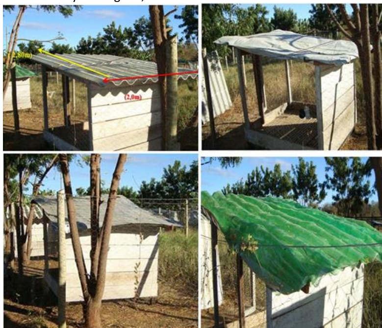
Figure 1 Roofing materials used for making the tiles: A- Fiber cement; B- Cardboard covered with double-sided canvas; C- Tetrapak® boxes and D- Tetrapak® boxes covered with PET bottles.
